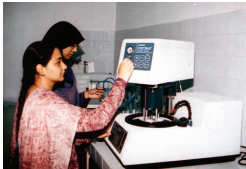
MSc students preparing samples using Metkon Polishing Machine in Materials testing laboratory
