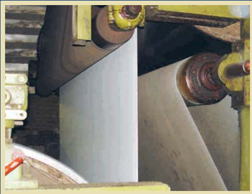
Paper sheet in the dryer section.
