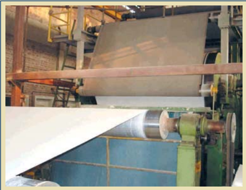
Sized paper sheet off the size press.
