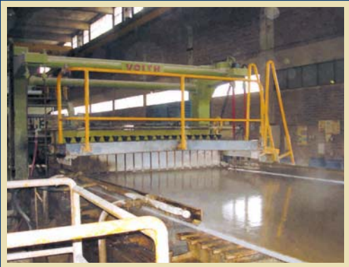
Wet paper web from head box to the wire.
