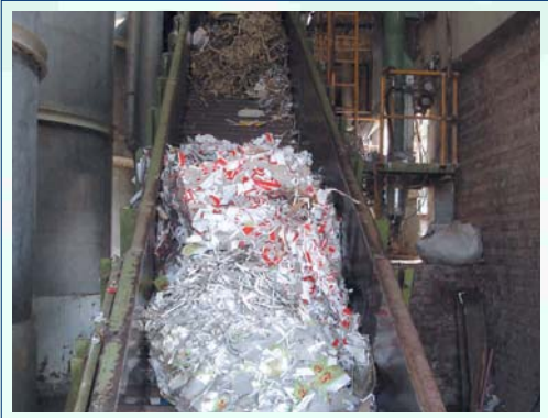
Waste paper on to the conveyor to pulper
