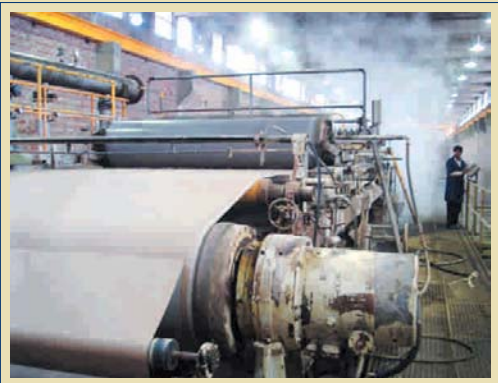
Wet paper to the dryer section.
