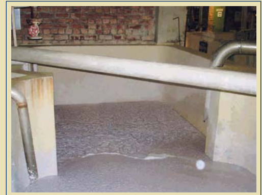
Recovered Fiber in the Mixing Chest.
