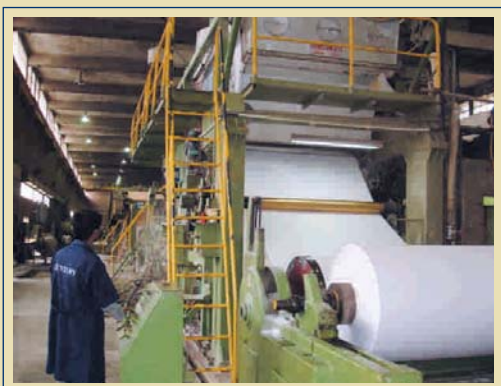
Formation of jumbo reel after coating.
