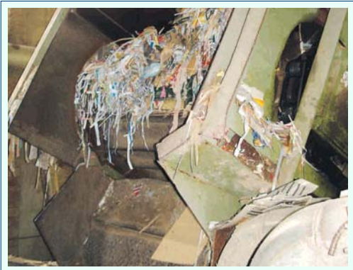
Waste paper feeding into the pulper
