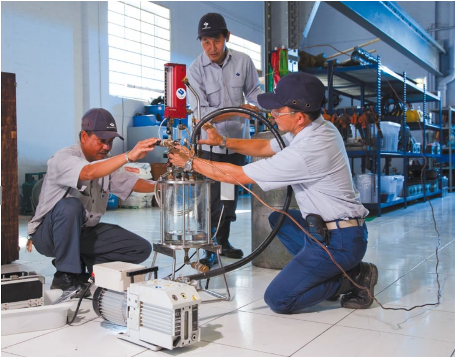
A team from the newly-formed Cable Jointing Unit carries out maintenance work on cable oil equipment.
