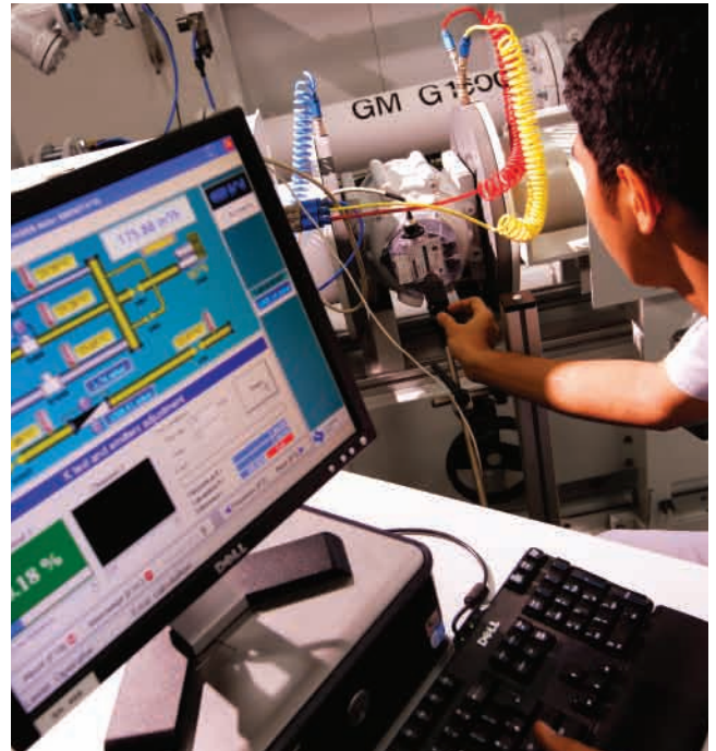
Calibration of gas meters being conducted at the Meter Laboratory.
