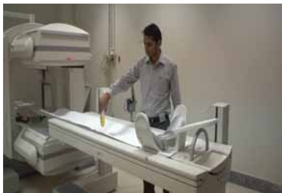
Radiation Survey in Gamma Camera Room
