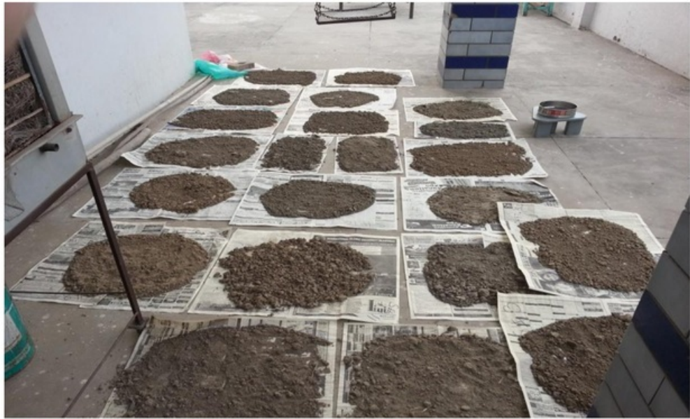
Fig.3.3. Sample preparation: Sample air drying and sieving
