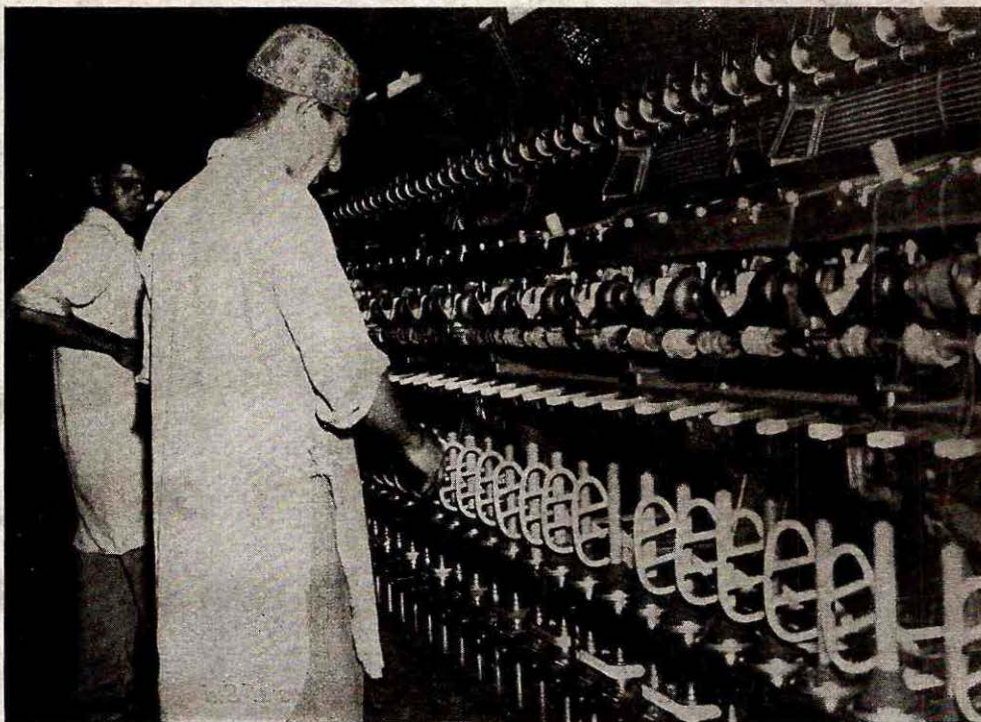
Ring Spindle in operation at the WPIDC's Harnai woollen mills, at Harnai in West Pakistan.
