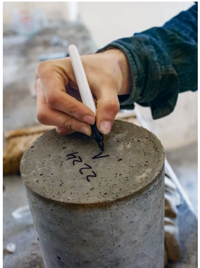
Samples for testing the mechanical strength of concrete.
