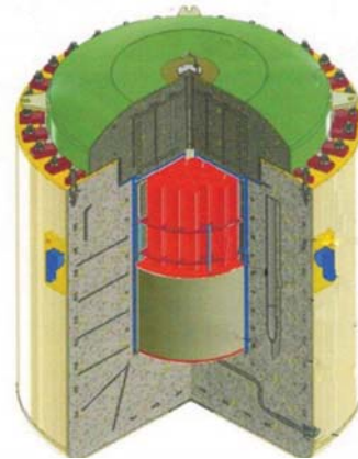
Schematic Design of Spent Nuclear Fuel Dry Storage Cask
