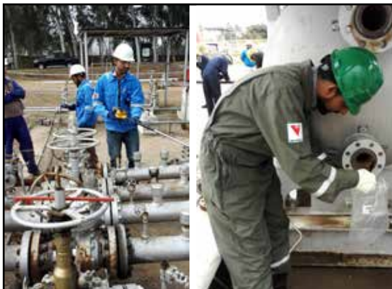
Radiation Survey and Sample Collection at NORM Producing Industries
