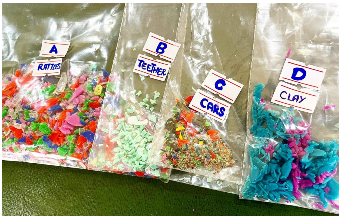
Fig 3.2. Prepared samples after crushing into small pieces of size of 0.5 cm.
