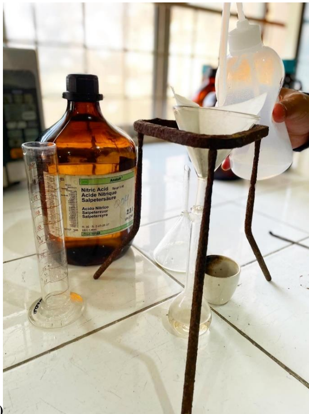
Fig 3.3. Samples during digestion and dilution
