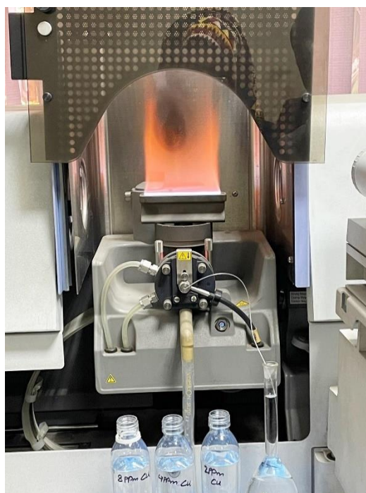
Fig 3.6: Blank solution run to calibrate the instrument
