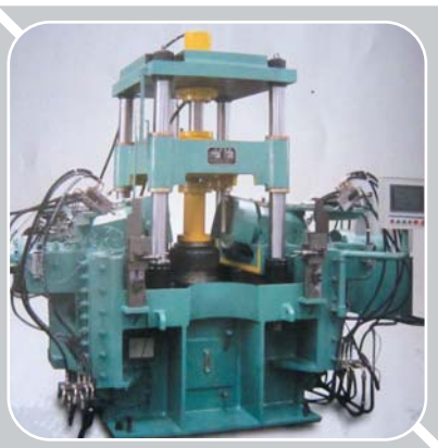
New Induction of Automobile Disc profile Forming Machine by Spinning Process
