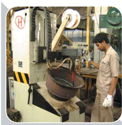
New Induction of CO2 Welding
