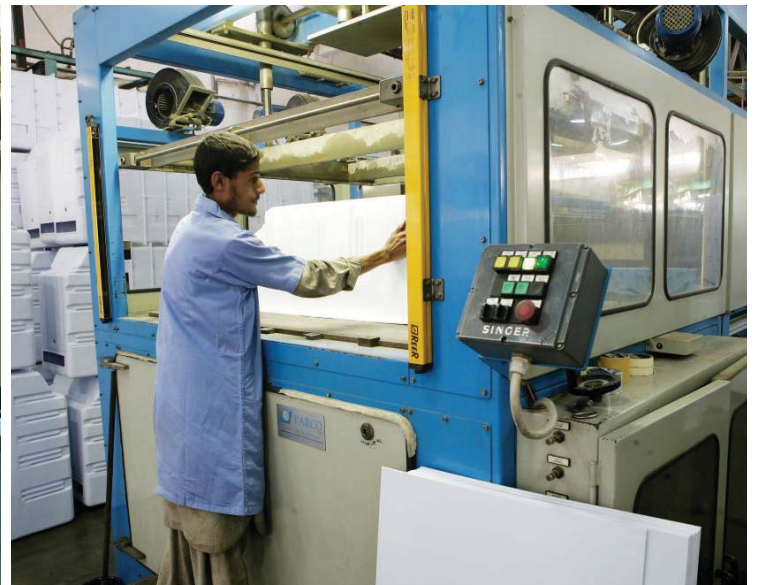
Vacuum forming section of the Refrigerator Plant.
