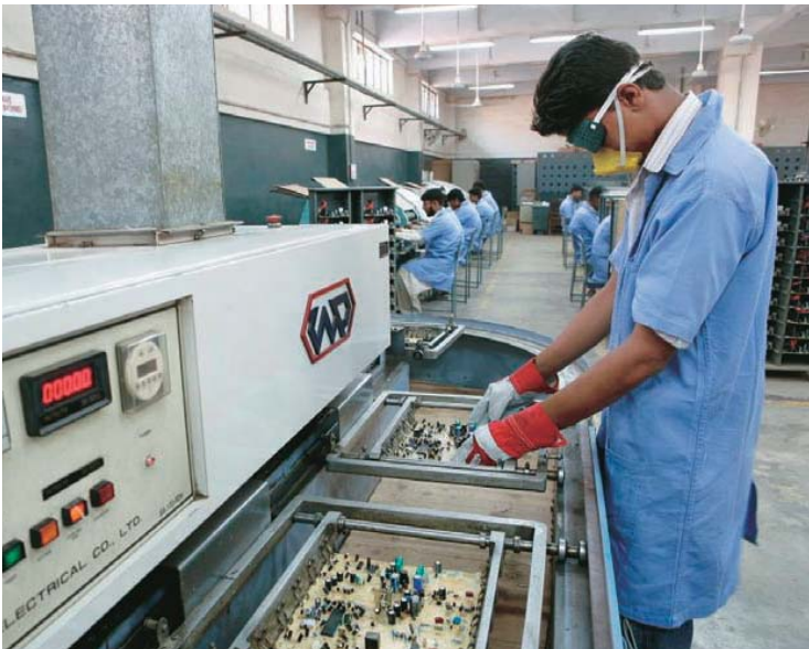
Dip soldering stage in CTV Assembly Plant
